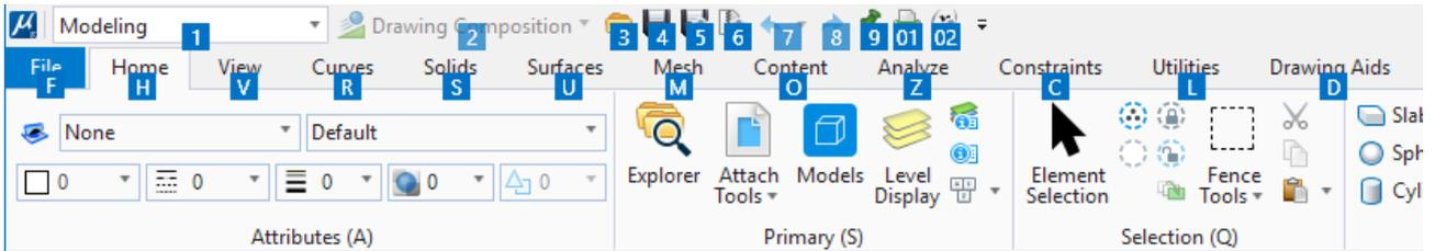
Press the appropriate letter to activate the desired Ribbon Tab or number (combination) to activate a QAT tool.
