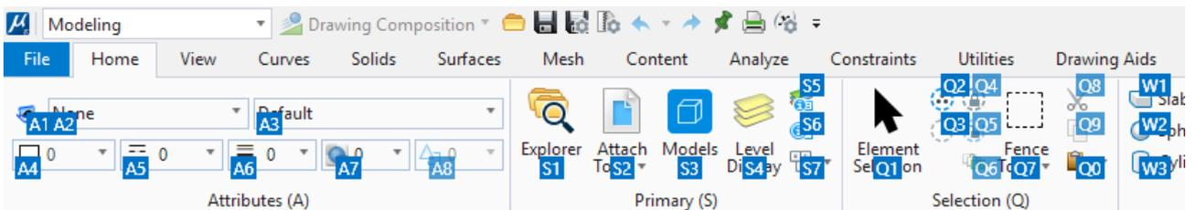
The KeyTips displayed in response to F3 have two conditions, those shown above are generated when Position Mapping is on, note how the KeyTips in each group start with the assigned Position Mapping letter followed by a sequential number (this is because the Auto-Generate KeyTips toggle is turned on and locked once Position mapping is on).
