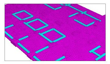
In the model shown in the above figure, the raft is modeled by connecting discrete individual foundations (footings or pile-caps). Beams are also modeled as connecting members between those individual foundations. Past versions of SACD were not able to identify these beams.
