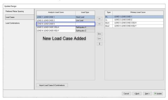
Load combinations to be considered can also be modified based on the load cases considered.
