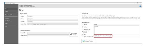
When the analysis file is read in RCDC and the beam module is selected, a new option named "Consider beams at Foundation level" will become available as highlighted in the above screenshot. The Y coordinate of that level is also displayed in the dialog box, and the user must select that to confirm that the beams are located at that level.
