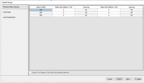
If any beams of width different than existing beam widths are available in the new analysis file, then, RCDC will update the above list of beam widths. Users will be able to change the rebar numbers for new widths only.
