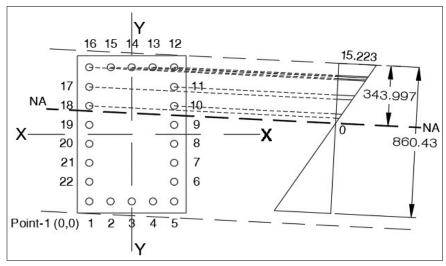
Compressive Stress at extreme edge of concret 15.22 N/sqmm =
