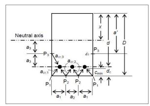
As the above process is iterative, For the Validation of this example, section capacity is calculated for a given column size and reinforcement arrangement and section capacity is calculated as per the available stress in the concrete and reinforcement.
