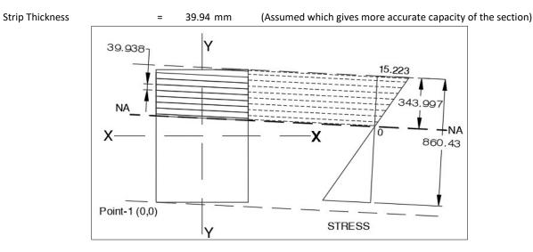
Compressive Stress at extreme edge of concret 15.22 N/sqmm =
