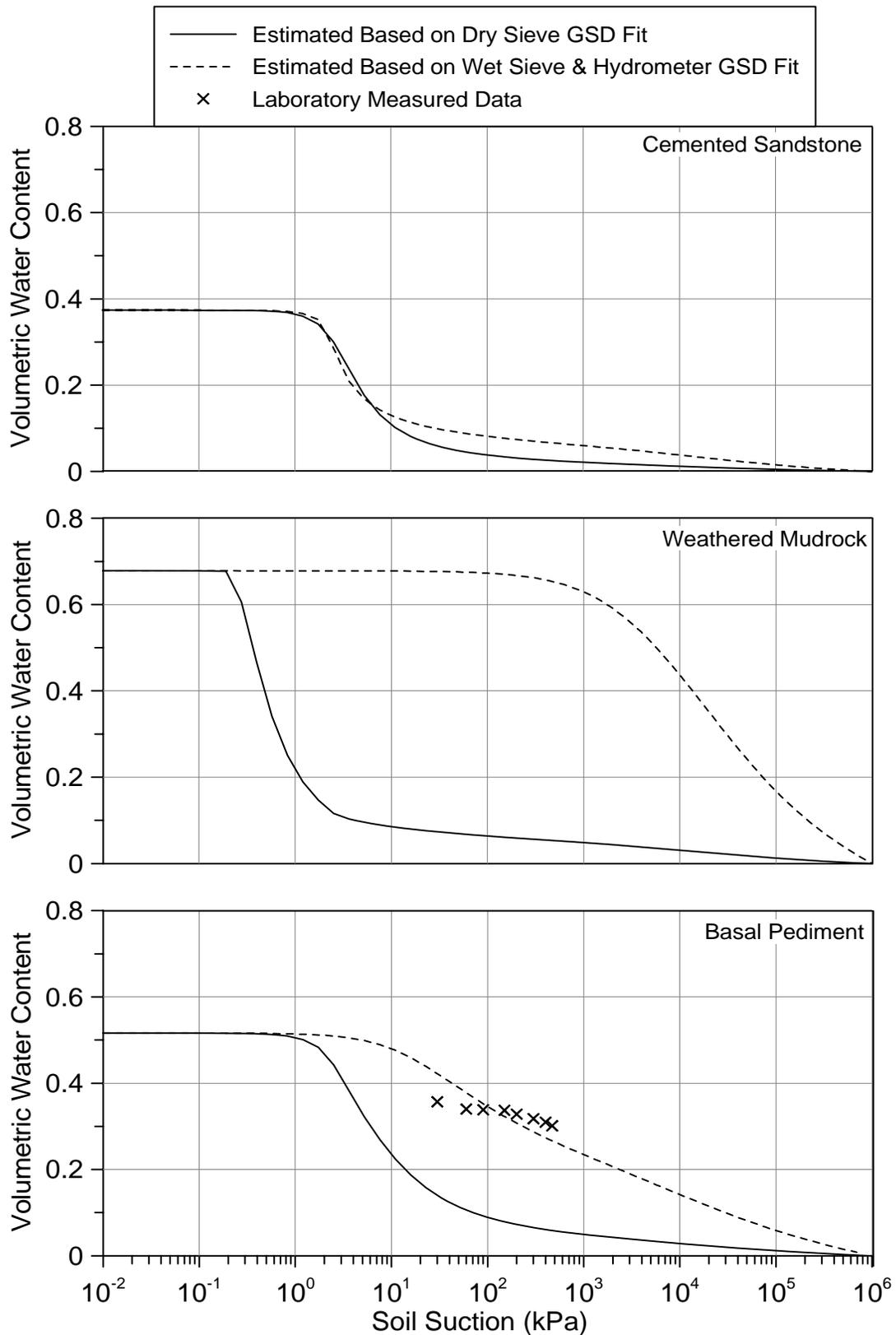
Figure 4: Soil water characteristic curves for the selected samples
