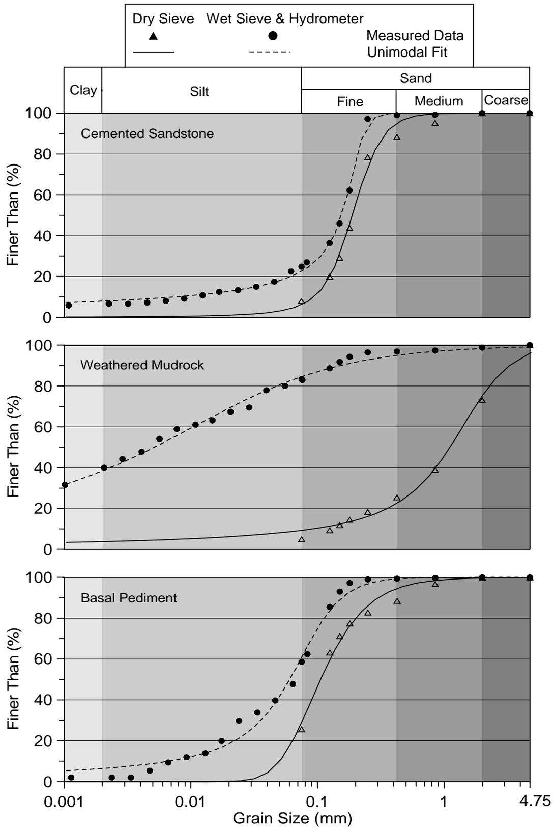
Figure 3: Grain size distribution for the selected samples
