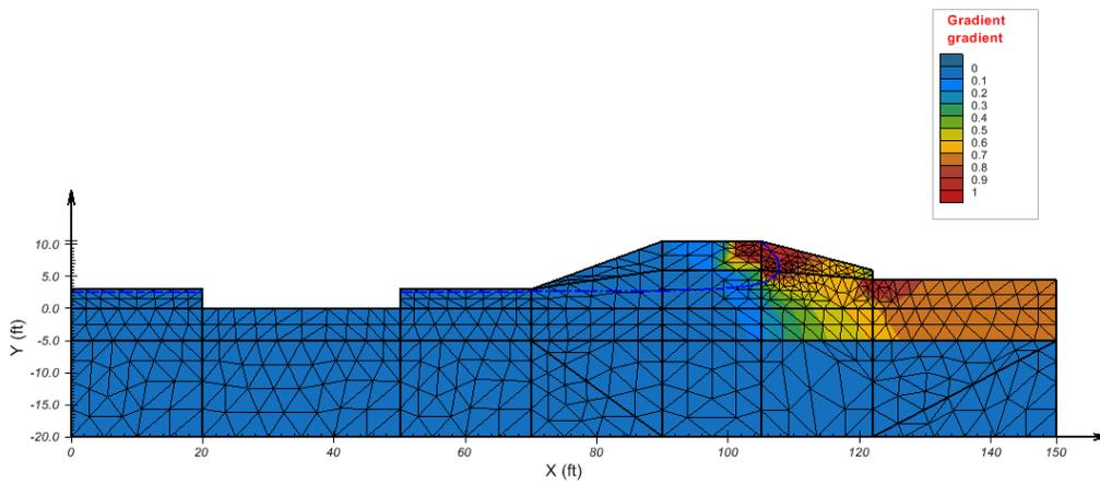
Figure 11: Critical gradients at the peak of the transient maximum design flood wave
