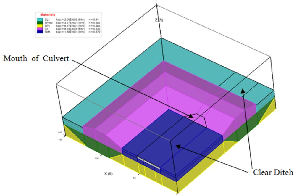
Figure 4: 3D Levee Intersection Geometry
