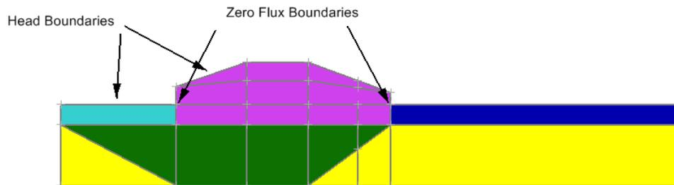
Figure 3: North-South Culvert Geometry (along Clear Ditch centerline). See cross-section B-B1 location in Figure 5.
