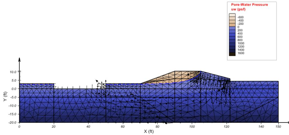
Figure 8: Pore-water pressure contours and flux vectors at the peak of the mean annual flood
