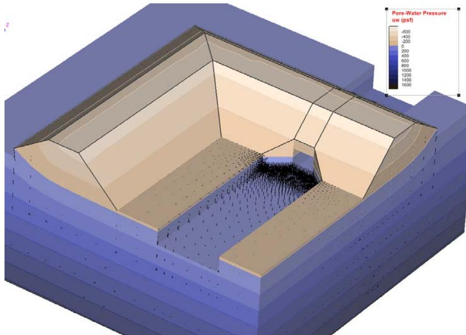
Figure 13: Pore-water pressure contours and flux vectors for the steady-state snowmelt flood wave, showing saturated (blue) and unsaturated zones (brown)
