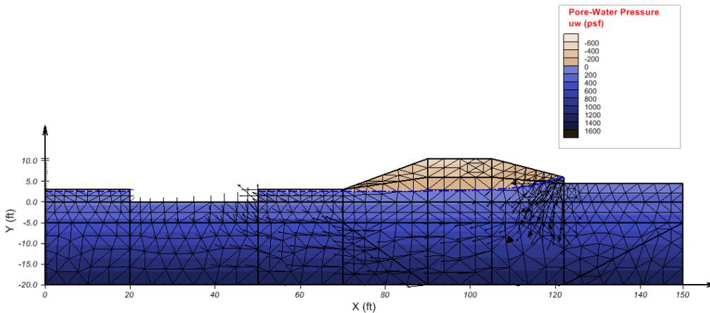
Figure 6: Pore-water pressure contours and flux vectors at the peak of the snowmelt flood wave
