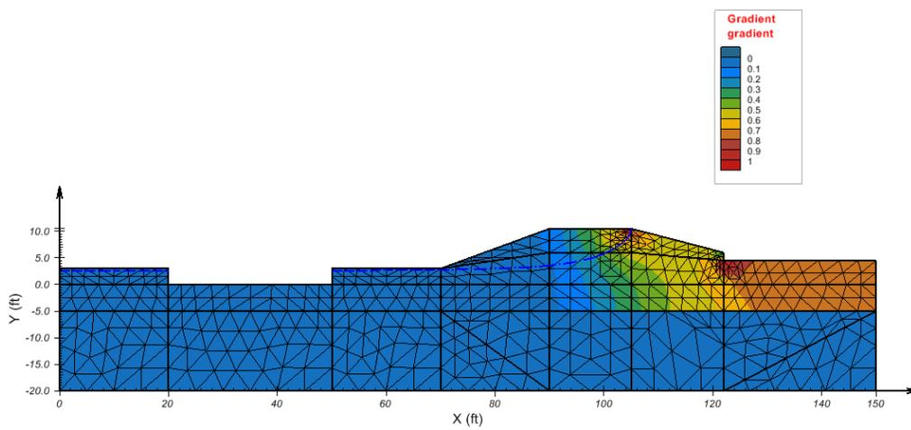
Figure 9: Gradients at the peak of the steady-state maximum design flood wave
