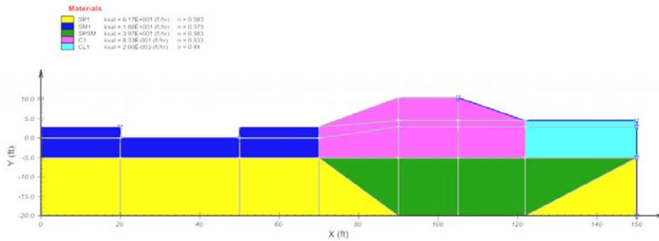
Figure 2: East-West 2D Cross Section. See cross-section A-A1 location in Figure 5.
