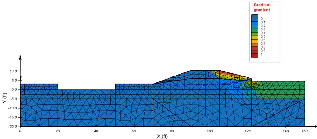
Figure 7: Gradients and flux vectors at the peak of the snowmelt flood wave
