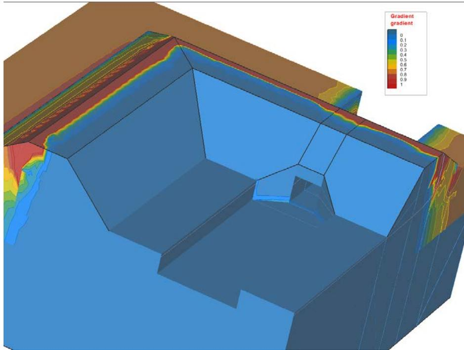
Figure 16 Critical gradients near the wing walls for the transient maximum design flood
