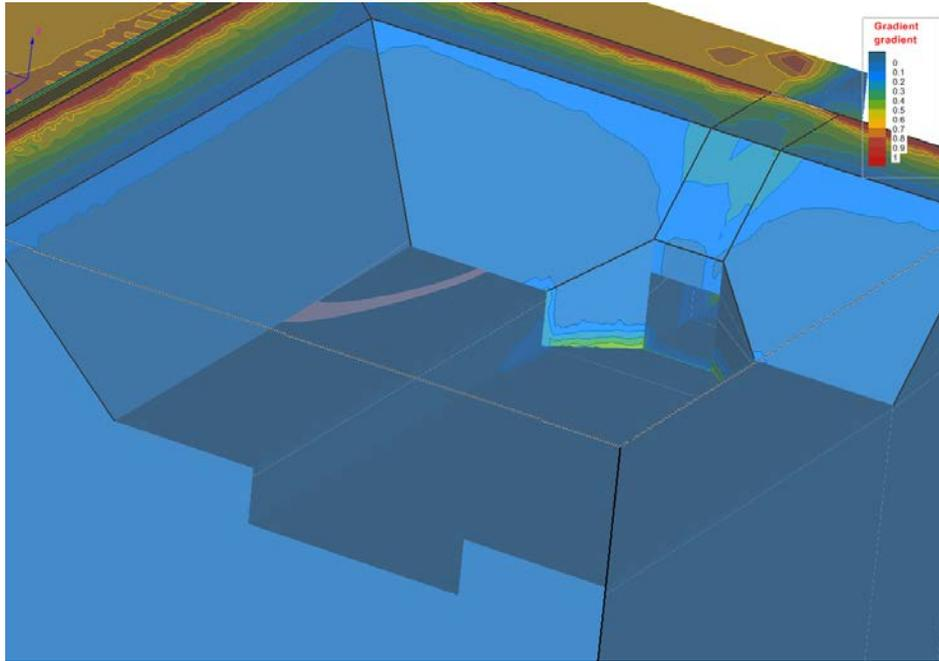
Figure 14: Critical gradients near the wing walls for the steady state maximum design flood
