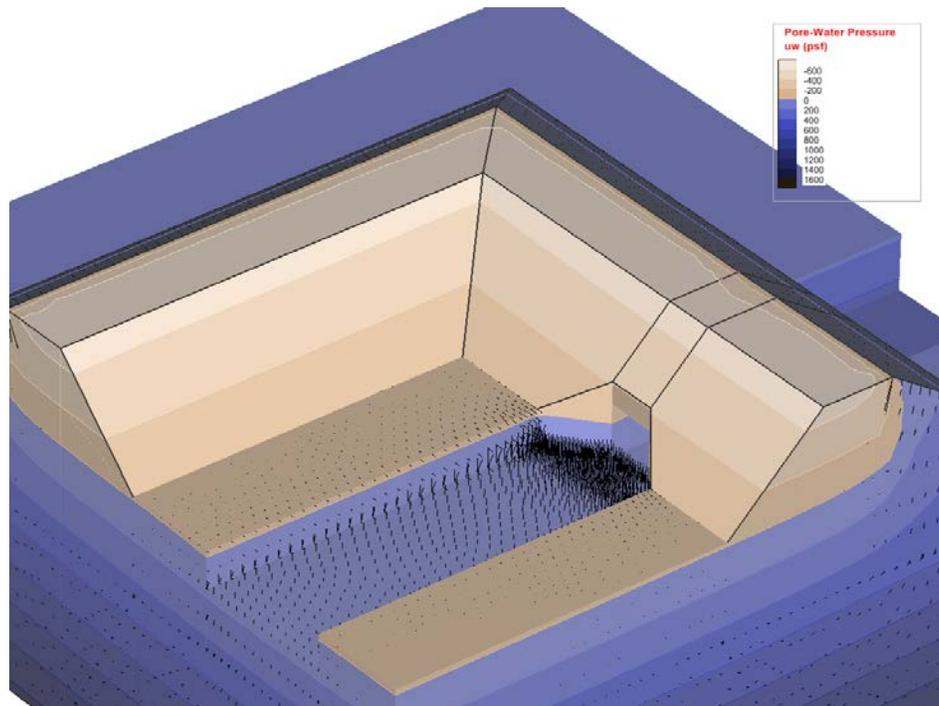
Figure 17: Pore-water pressure contours and flux vectors for the transient maximum design flood, showing saturated (blue) and unsaturated zones (brown)
