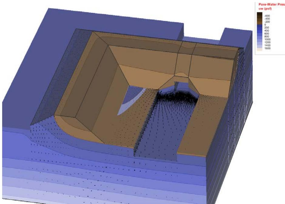
Figure 15: Pore-water pressure contours and flux vectors for the steady-state maximum design flood, showing saturated (blue) and unsaturated zones (brown)
