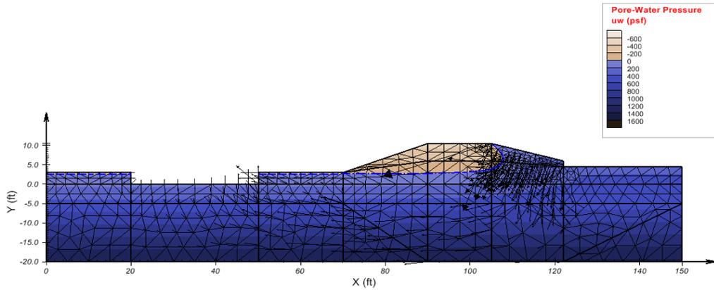
Figure 10: Pore-water pressure contours and flux vectors at the peak of the transient maximum design flood wave
