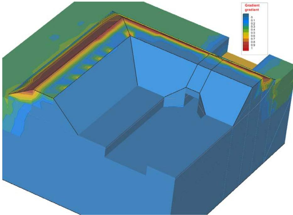
Figure 12 Critical gradients near the wing walls for the steady-state snowmelt flood wave
