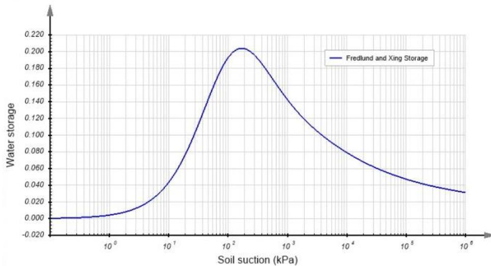
Figure 6. Water storage function for the artificial clayey silt
