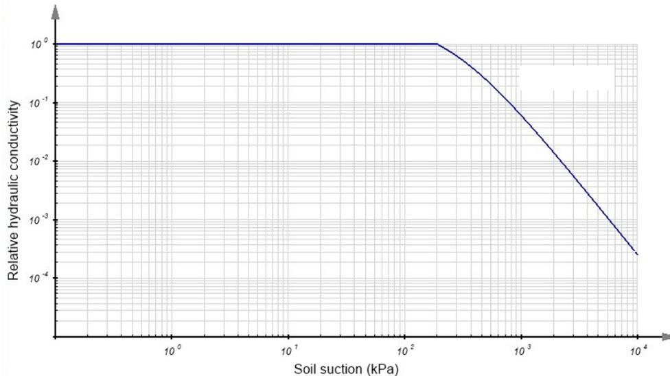
Figure 8. Permeability function for the artificial clayey silt
