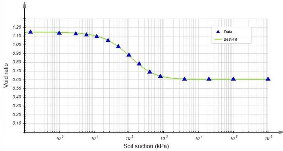
Figure 4. Void ratio SWCC for the artificial Clayey Silt
