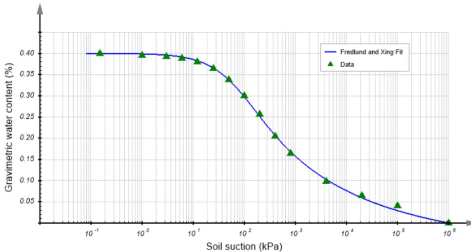
Figure 2. Gravimetric water content versus soil suction for artificial clayey silt
