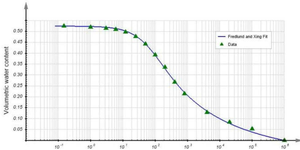
Figure 5. Volumetric water content SWCC for the Artificial Clayey Silt
