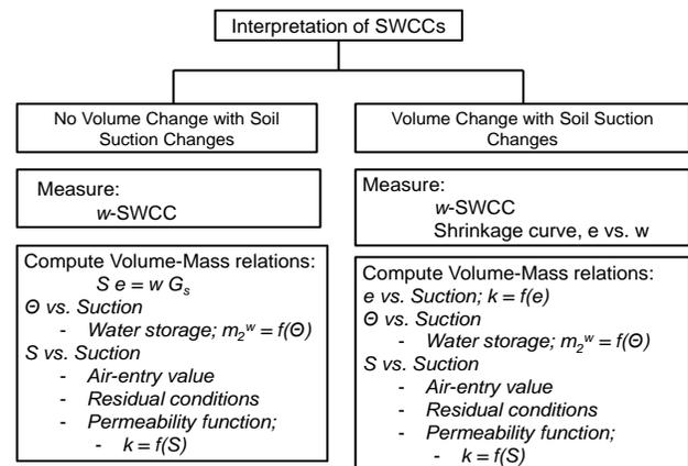
Figure 1. Measurements required for the calculation of USPFs for "volume change" and "no volume change" soils as soil suction is increased
