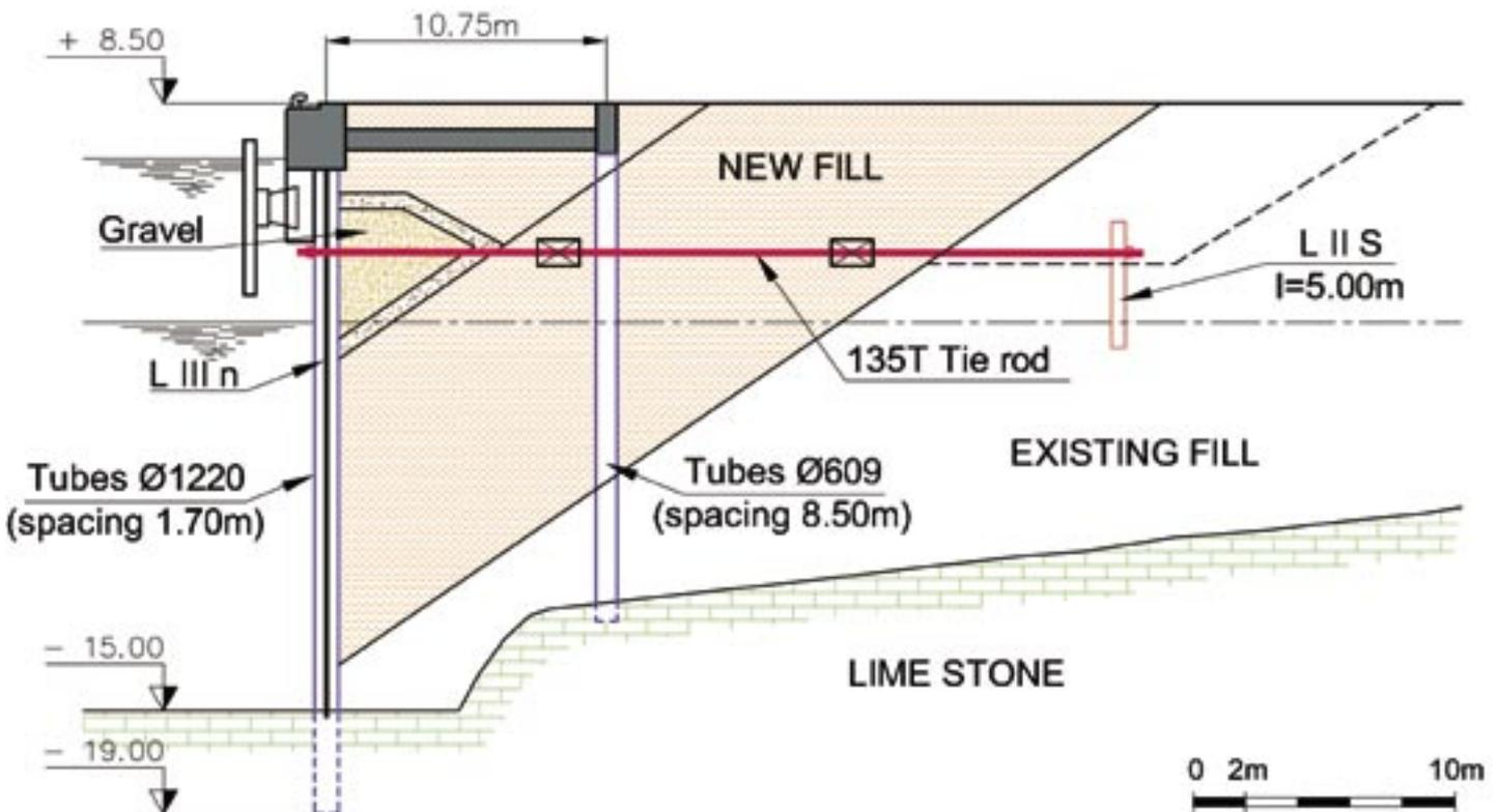
Figure 1: Schematic quay cross section (CM: datum at lowest astronomical tide)
