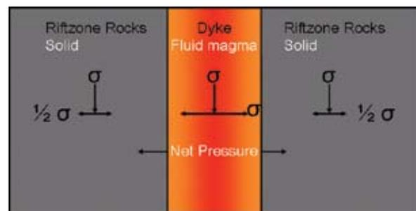
Figure 3 Illustration of the stress difference in a fluid and in a rock mass
