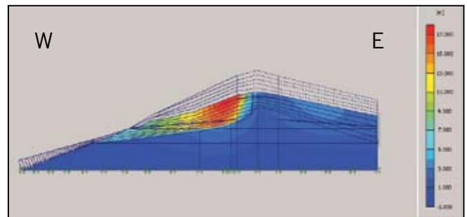
Figure 5. Total displacements due to historical growth only. The plane of weakness is formed by a sequence of Post Collapse Sediments.
