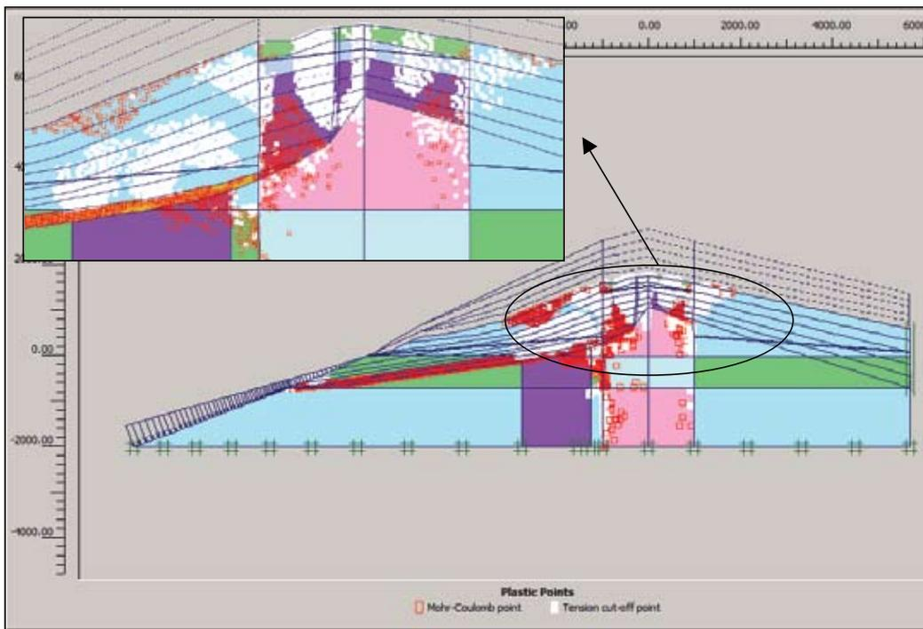
Figure 6 Failure points in the riftzone as a result of thermal pore pressures. The thermal pore pressures form due to heat radiation of deep seated magma intrusions.
