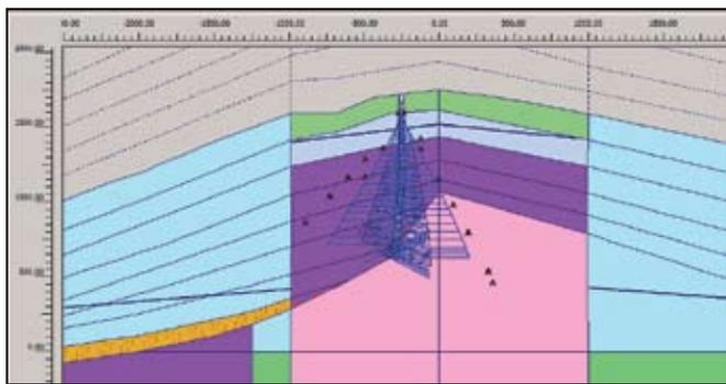
Figure 4. Layout of the prescribed load system that simulates a magmatic dyke pressure
