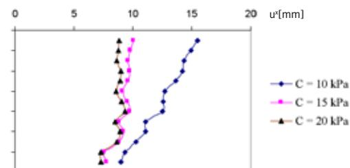
Figure 5 Variation of maximum horizontal displacement of nails with depth
