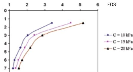
Figure 3 Variation of factor of safety with the depth of excavation
