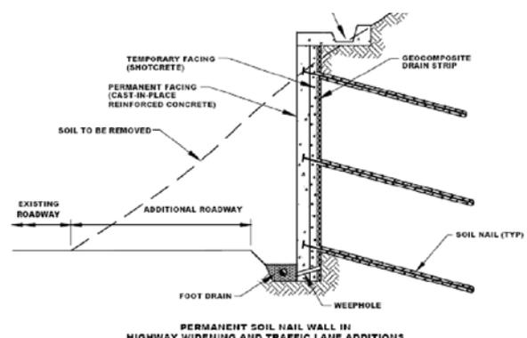
Figure 1. Examples of use of soil nail walls in temporary and permanent cut applications.
