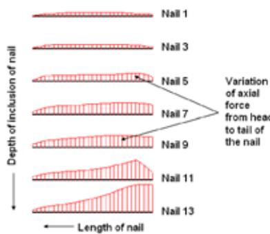
Figure 7 Pattern of variation of axial force along nail length (alternate nail from top shown)
