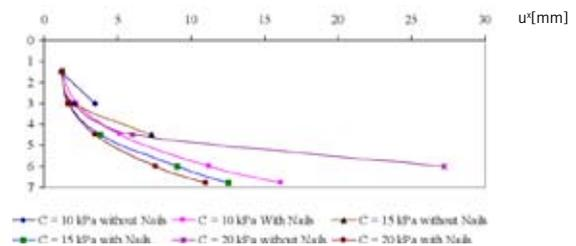
Figure 4 Variation of horizontal displacement of vertical cut with depth of excavation
