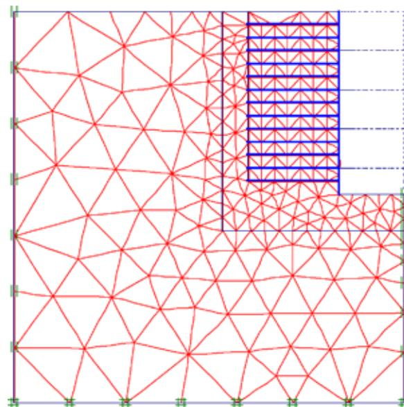
Figure 2 Finite element model for the soil nailed wall
