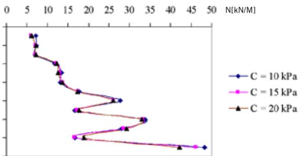
Figure 6 Variation of maximum axial force in nails with depth
