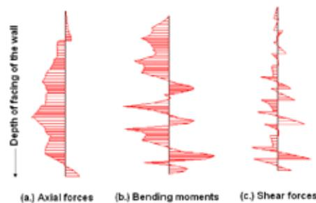
Figure 8 Variations of axial forces, bending moments and shear forces in facing elements
