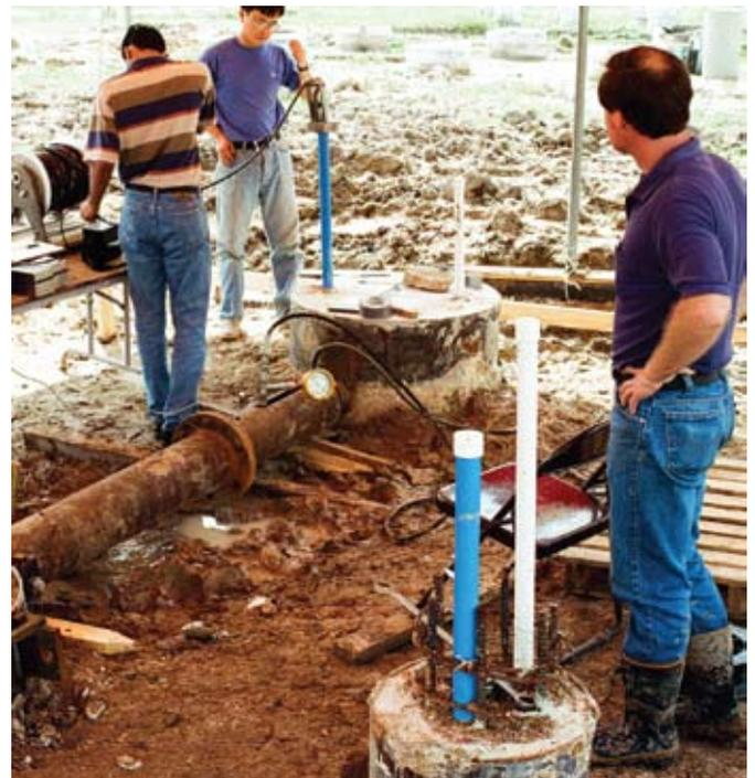
Photo 1: Load Testing a 0.91 m Diameter ACIP Pile
