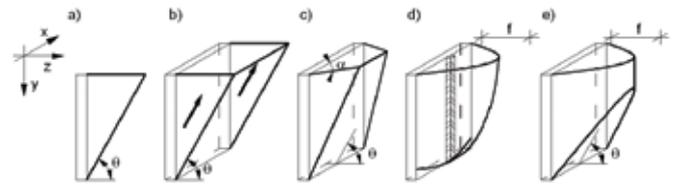
Figure 1: Shapes of the sliding wedges studied by: a) Nash and Johns (2D); b) Morgenstern and Amir-Tahmasseb; c) Washbourne; d) Tsai and Chang; e) Piaskowski and Kowalewski.
