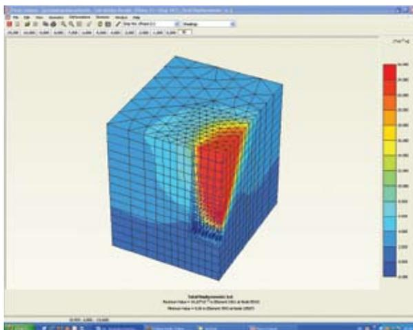
Figure 4a: The 3D total displacements (at failure).
