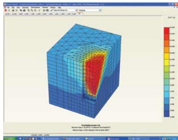
Figure 7a: The 3D soil displacements (at failure).
