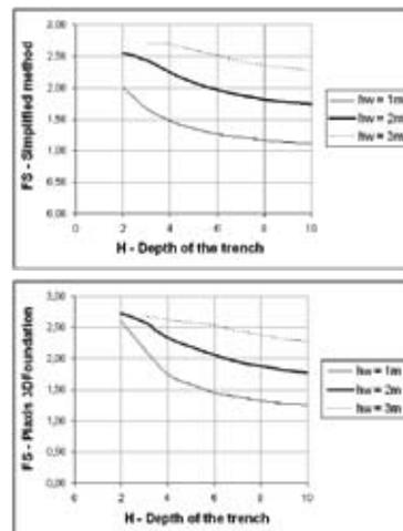
Figure 5: Comparison of two calculation methods in term of the factors of safety FS.
