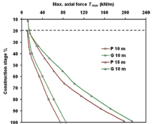
Figure 5: Development of maximum axial force with construction stage
