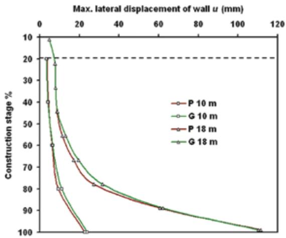
Figure 4: Trend of lateral displacements with construction stage
