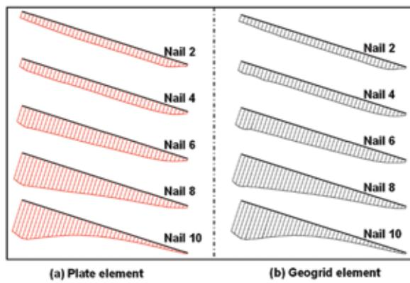
Figure 6: Variation of axial force along nail length (10 m high soil nail wall)
