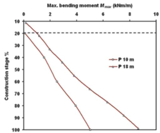
Figure 7: Development of maximum bending moment with construction stage
