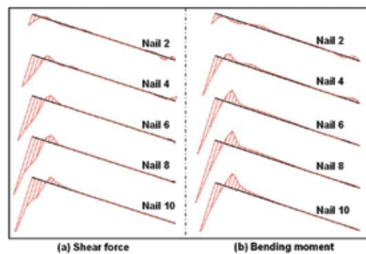
Figure 9: Variation of shear force and bending moment along nail length (10 m high soil nail wall)
