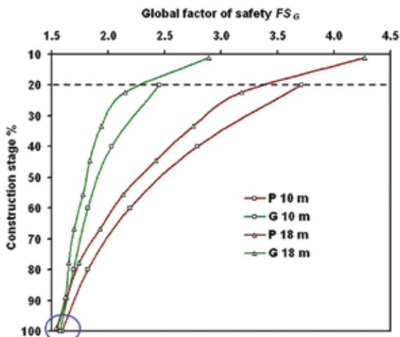
Figure 3: Trend of global factor of safety with construction stage
