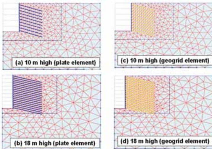
Figure 2: Simulated soil nail walls using PLAXIS 2D
