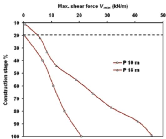
Figure 8: Development of maximum shear force with construction stage
