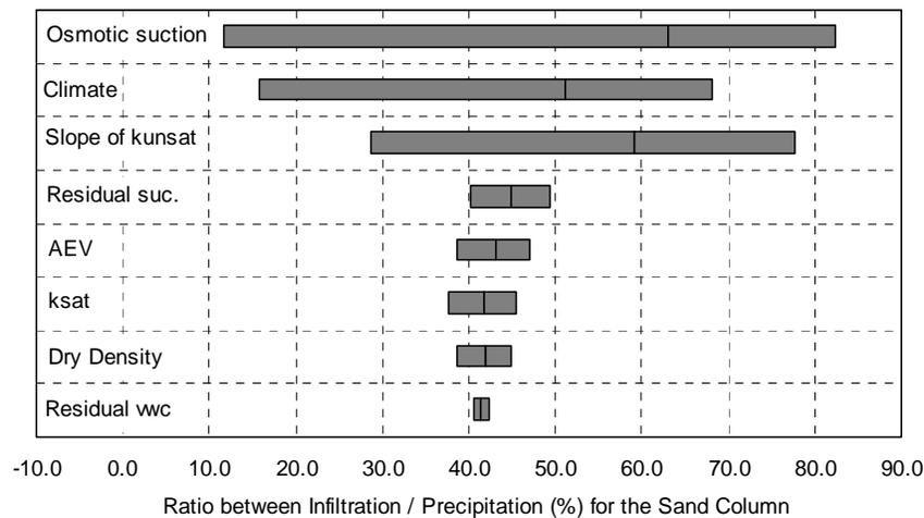
**FIG. 4. Tornado diagram illustrating the influence of various soil input parameters on infiltration.**
