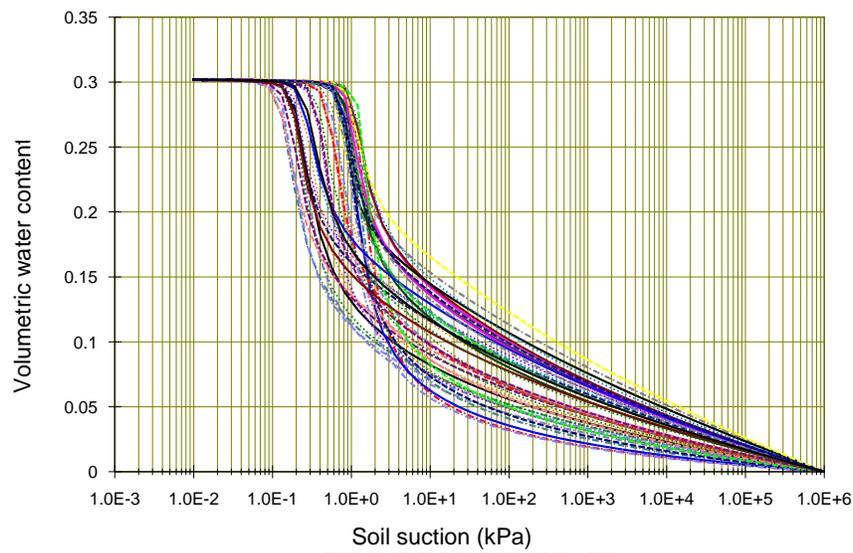
**FIG. 2. Group of theoretically estimated soil-water characteristic curves based on grain-size distributions**
