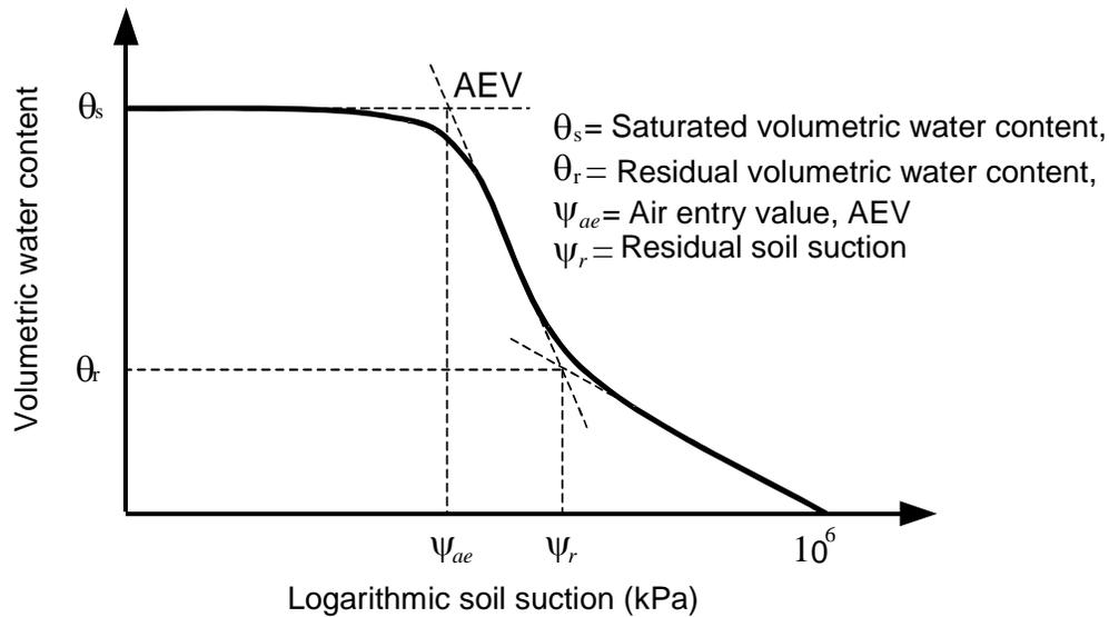
**FIG. 1. Conceptual model of physically realistic parameters to represent the soil-water characteristic curve.**
