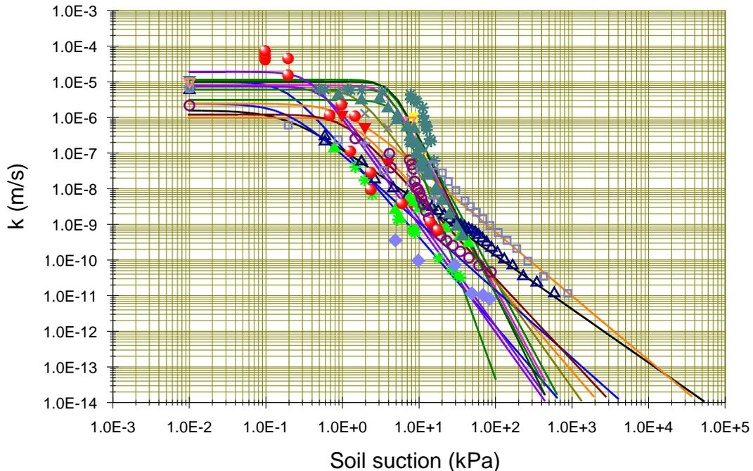
**FIG. 3. Group of hydraulic conductivity unsaturated curves matching the grain-size distributions.**
