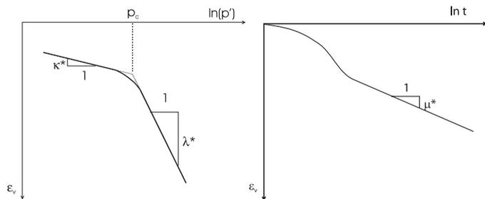
Figure 1: Graph of volumetric strain vs. natural logarithm of mean stress
