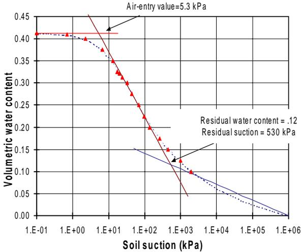
Figure 5 Results of the construction technique for a Silt Loam (from van Dam et al. 1992) (SoilVision soil #133)
