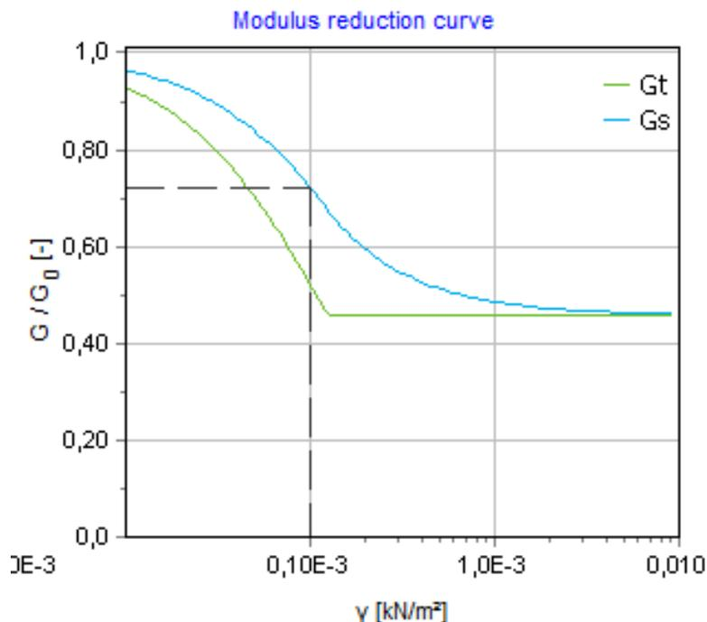
Figure 213: Modulus reduction curve for the lower sand layer
