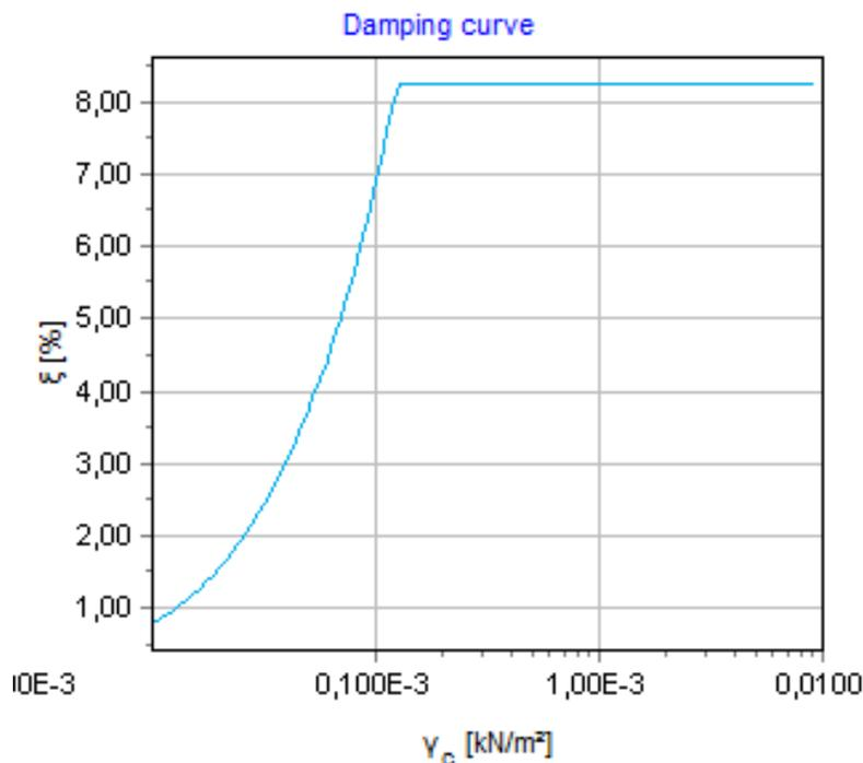
Figure 215: Damping curve for the lower sand layer
