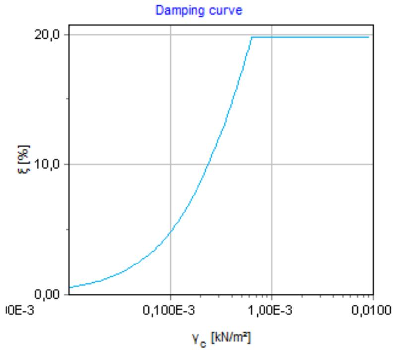
Figure 214: Damping curve for the upper sand layer
