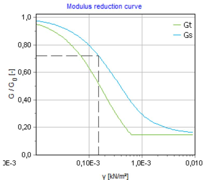
Figure 212: Modulus reduction curves for the upper sand layer
