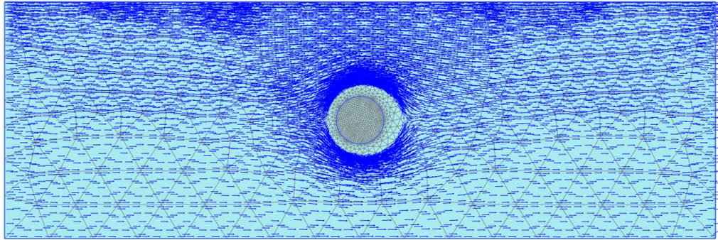
Figure 249: Groundwater flow field after 180 days
