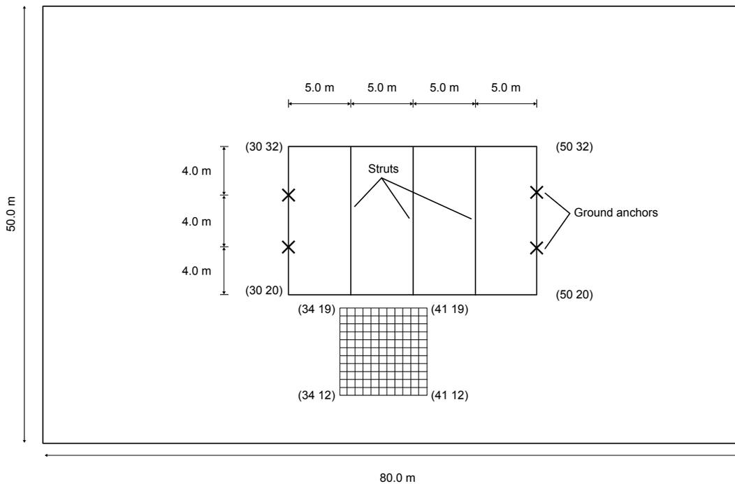
Figure 29: Top view of the excavation pit
