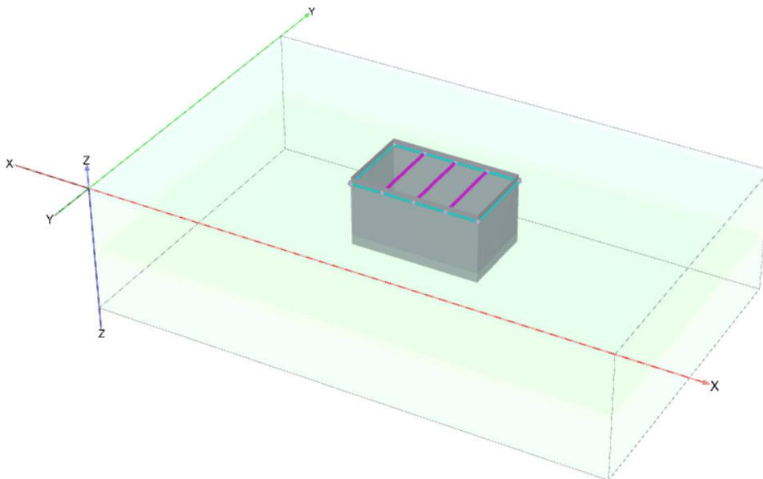
Figure 31: Visualization of struts and walings - Structures mode
