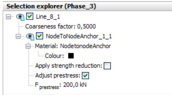
Figure 33: Node-to-node anchor in the Selection explorer
