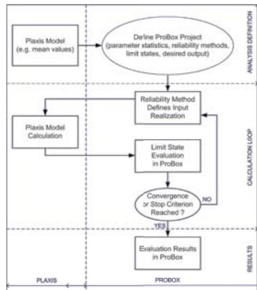
Figure 4. Coupling Scheme ProBox-Plaxis
