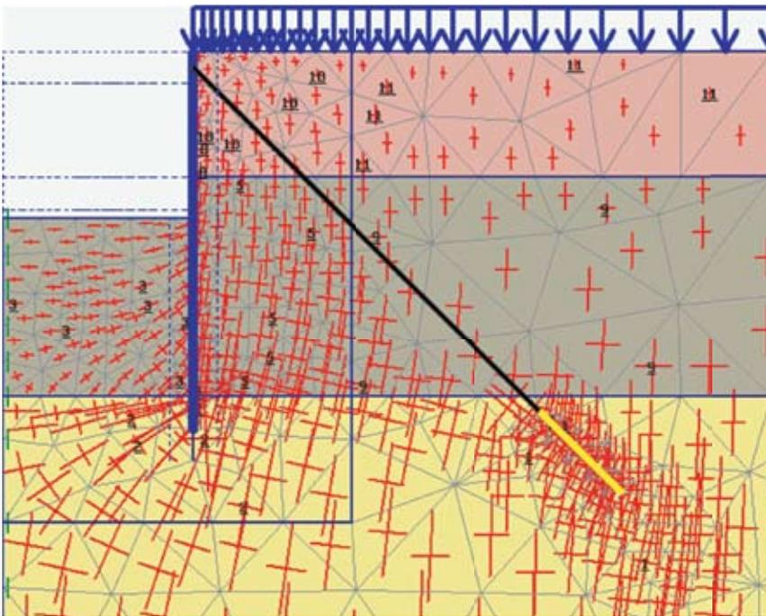
Figure 7. Principal Effective Stresses (Design Point Sheet Pile Failure)
