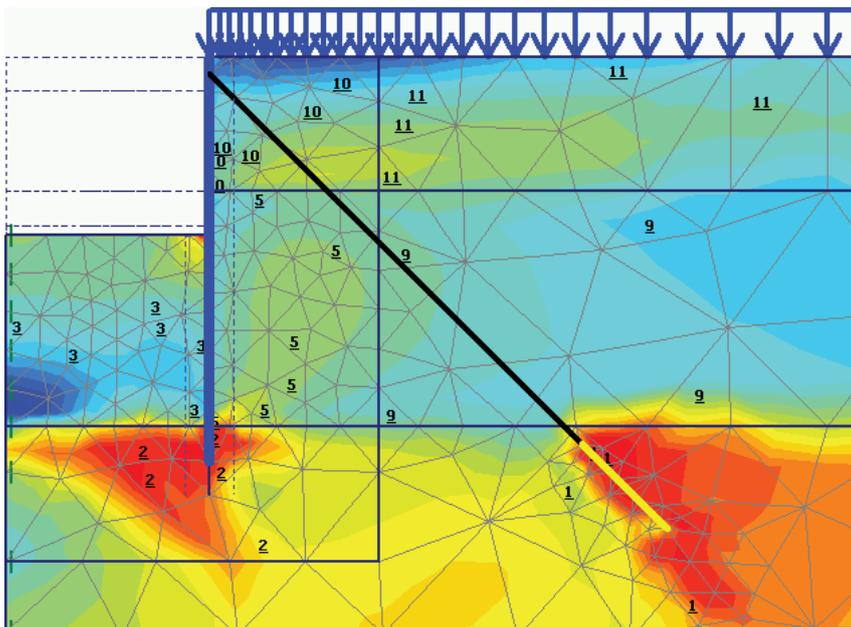
Figure 8. Relative Shear (Design Point Sheet Pile Failure)
