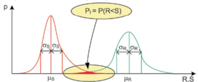
Figure 2. Partial Safety Factors vs. Fully Probabilistic
