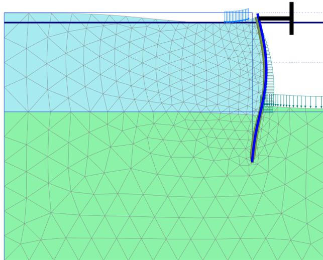
Figure 39: Deformed mesh after the third excavation stage
