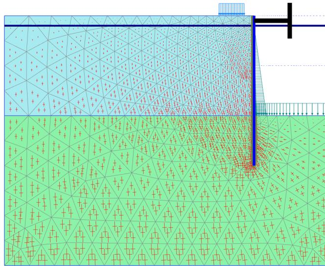
Figure 40: Principal stresses after excavation
