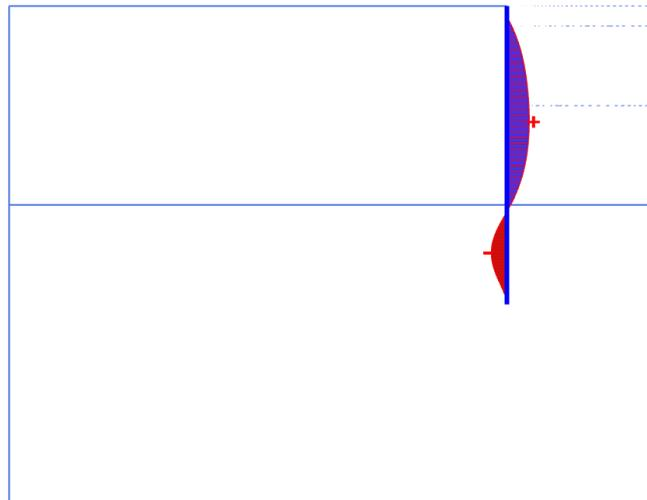
Figure 41: Bending moments in the wall
