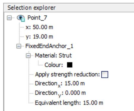
Figure 33: Parameters for fixed-end anchors in the Selection explorer
