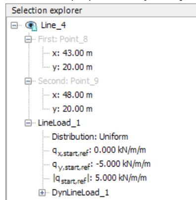
Figure 34: Components of the distributed load in the Selection explorer
