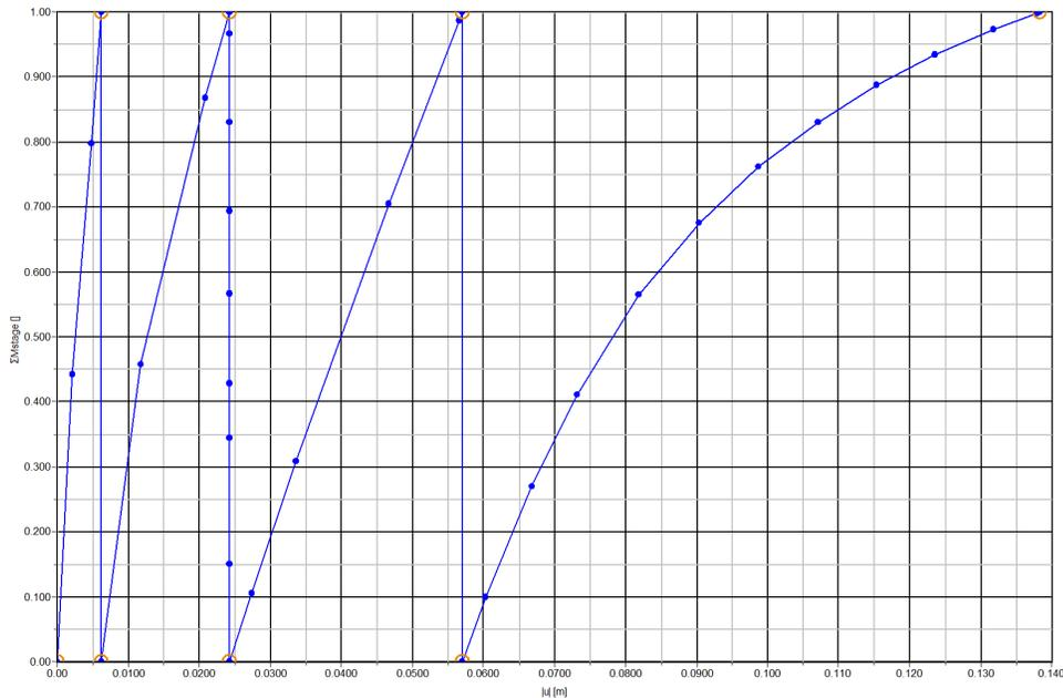
Figure 42: Load-displacement curve of deflection of wall
