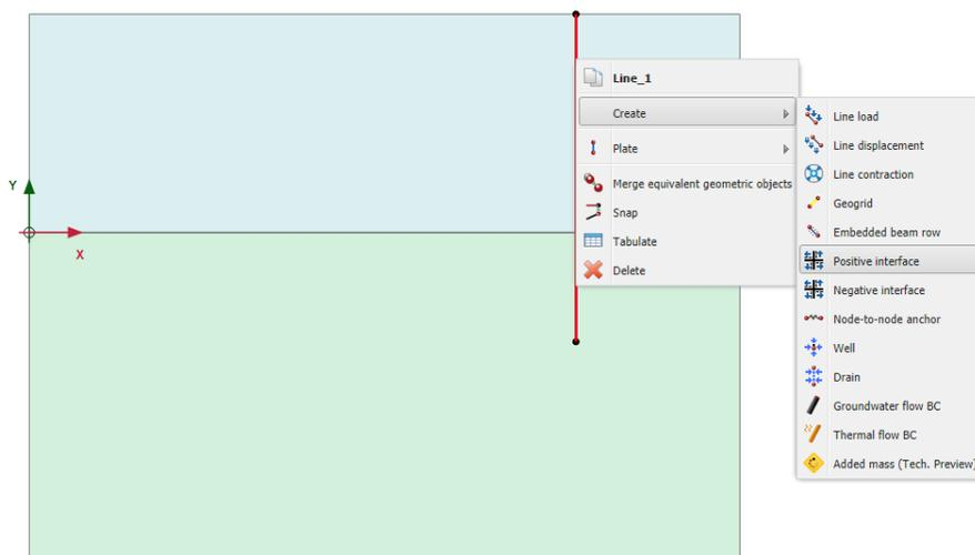
Figure 32: Positive interface assignment to existing geometry
