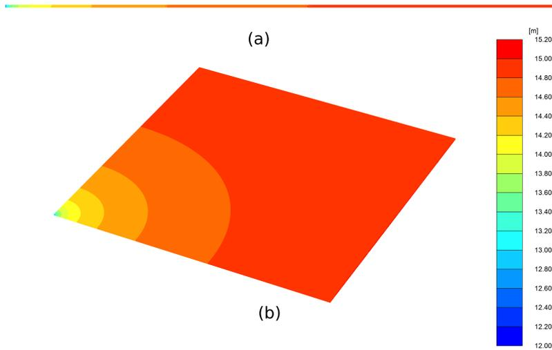
Figure 3 Groundwater head at steady-state conditions in PLAXIS 2D (a) and PLAXIS 3D (b)
