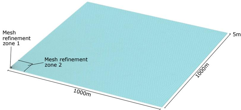
Figure 2 Model geometry and generated mesh (PLAXIS 3D)
