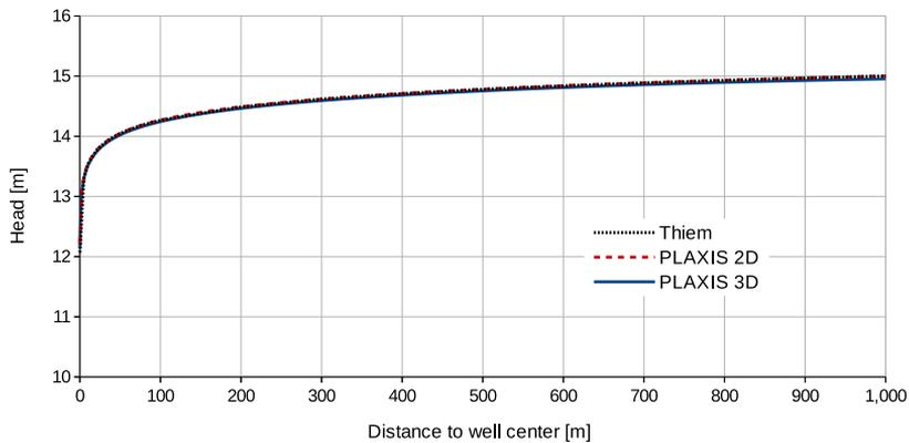
Figure 6 Head variation over distance from the well center at steady-state conditions
