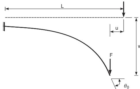
Figure 1 True deformation of elastic cantilever beam
