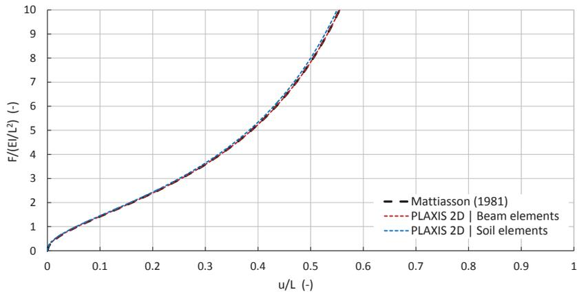
Figure 5 Variation of normalized load with horizontal displacement
