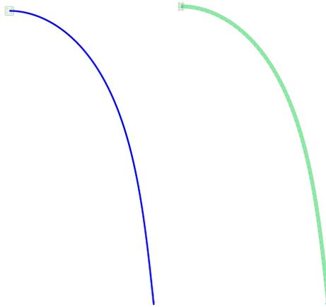
Figure 3 Deformed mesh (true scale) in case of beam elements (left) and soil elements (right)
