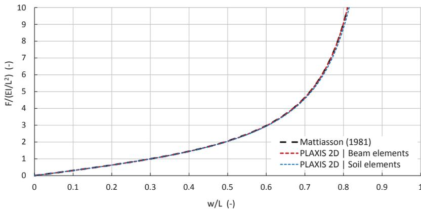
Figure 4 Variation of normalized load with vertical displacement
