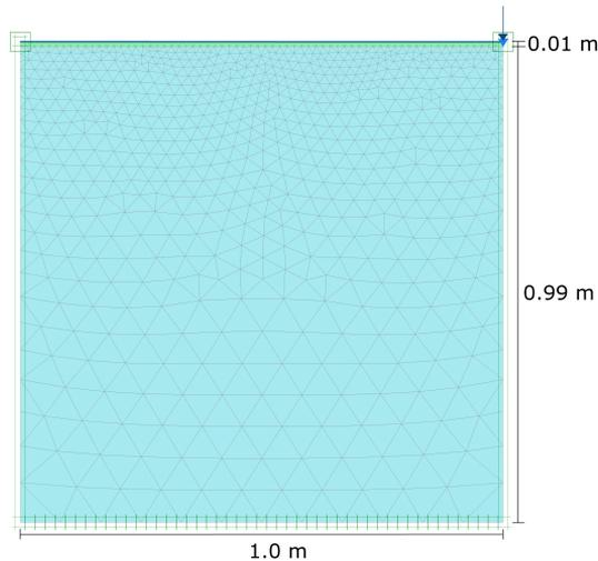
Figure 2 Model geometry and finite element mesh
