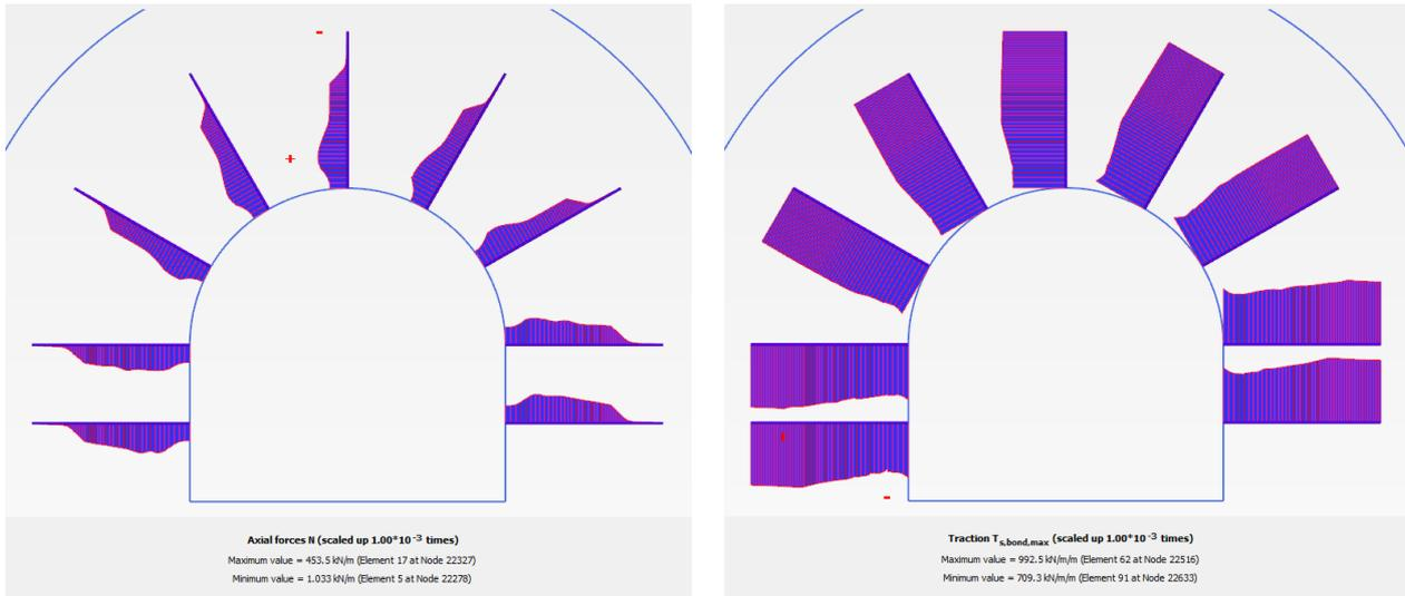
Figure 3.4: Excavation completion: axial forces on grouted cable bolts (left) and bond strength limit (right).
