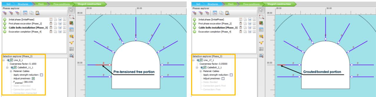
Figure 3.1: Cable bolt installation: pre-tensioned free portion (left) and grouted/bonded portion (right). Geometry of the tunnel
