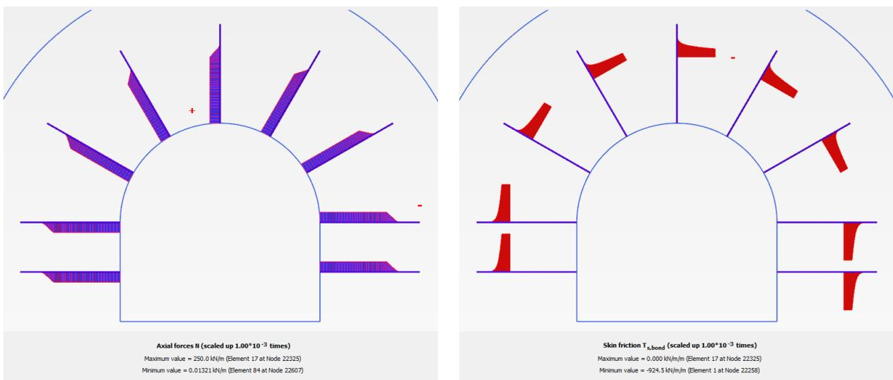
Figure 3.3: Cable bolt installation: pre-tension force on unbonded part (left) and bond strength mobilization on grouted part (right).
