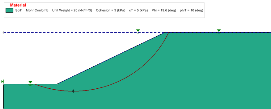
Figure 133 Geometry of the simple slope used for rapid drawdown calculations
