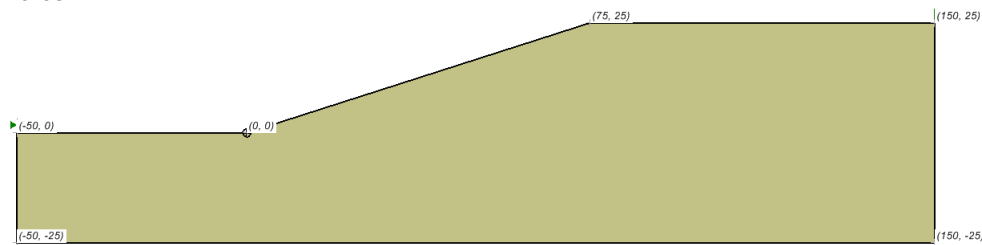
Figure 114 Geometry of the Loukidis Seismic Coefficient model (VS_62_Dry)
