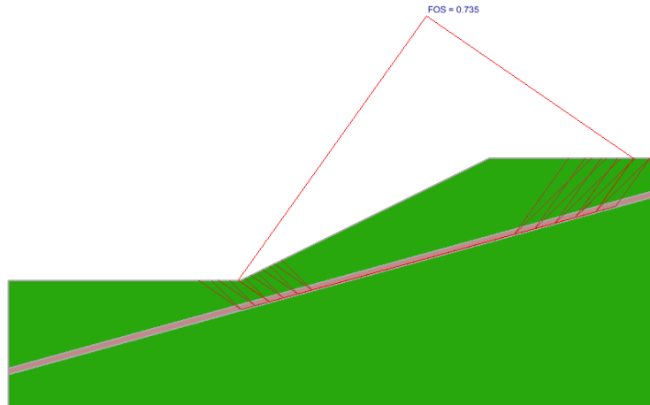
Figure 32 Solution using the Spencer Method
