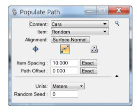
This mode of the tool will place items at specified points along a path. Once the path has been selected prompts to select the start and end points of placement will be displayed followed by a data point to accept the placement.
