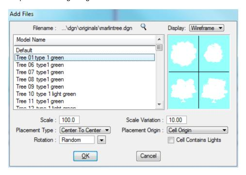
This dialog allows the user to open a .dgn,.cel,.dgnlib etc. file and select a series of models within that file for use as items to place.
