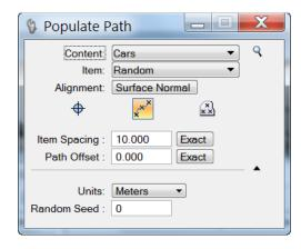
This mode of the tool will fill a shape with items based on the criteria specified in the tool. Simply identify the shape to be populated (or if populating a fence is required then check the "Use Fence" option). Then items will be placed on the surface within the area.
