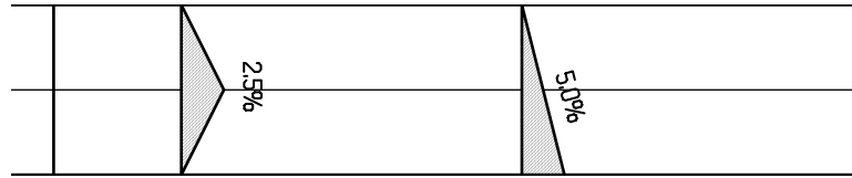
Figure 3 - 143 Crossfall annotation at points of change
