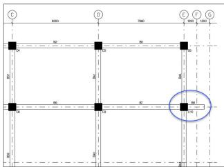
B8 is ignored in the joint check of column C10 at that level.
