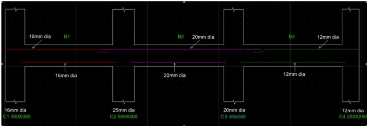
Detailing Option: Min Diameter
