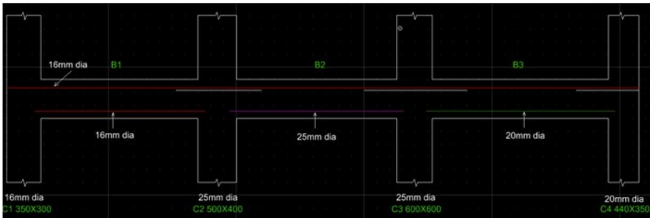
For various options of redesign and re-detailing, the list of rebar that would be available would be as per restrictions of the adjacent column size.
