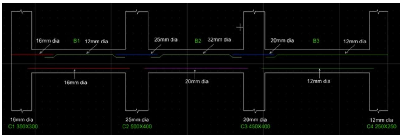
Detailing Option: Max Diameter
