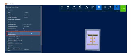
This will enable the friction calculation which can be calculated just for the plate or Include it in the anchors shear capacity.
