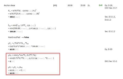
Finally, shear can also be resisted by a shear lug. If this is the case you need to check the option
