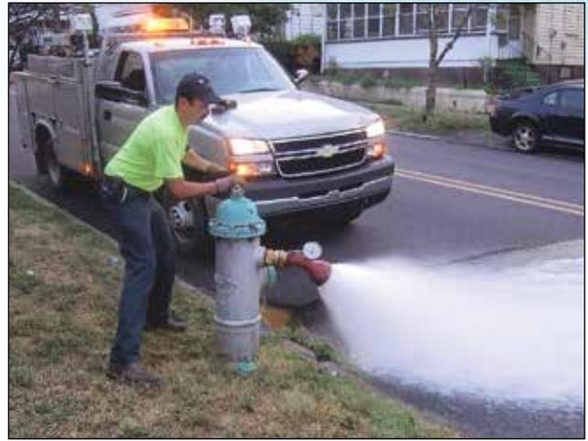
**Step 1:** Use data when the hydraulic grade line is relatively flat to identify errors and adjust pressure zone boundary valves, elevations, tank water levels, pressure-reducing valve settings, and other boundary conditions (left). **Step 2:** Conduct hydrant flow tests to provide increased velocity and head loss and make it easier to identify problems with roughness and demands (right). *Source: Thomas Walski*
